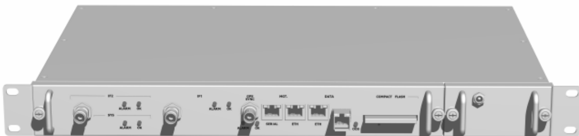
Figure 1: Indoor Unit IDU StarMAX™ 4120 Dual Sector Base Station
